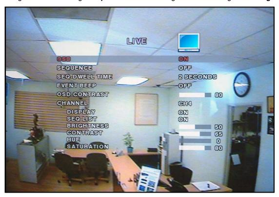
Figure 3.2.1. Live Mode Setup Screen
