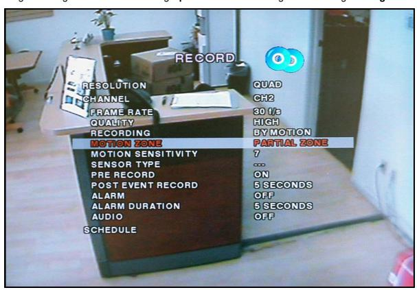
Figure 3.3.1. Recording Mode Set-up Screen
