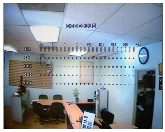
Figure 3.3.3. Recording Schedule Set-up Screen
