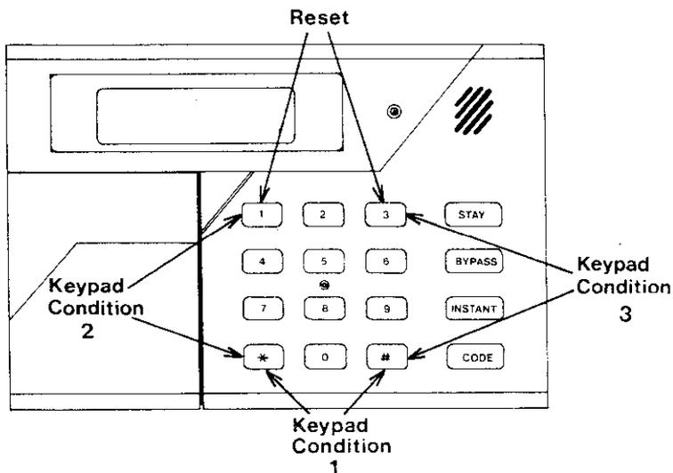
Conditions can be initiated directly through the keypad for various auxiliary conditions. These capabilities will be defined by your installer for conditions such as PANIC, FIRE, or AUXILIARY. The keypad conditions are active 24 hours a day, whether the system is armed or disarmed.
