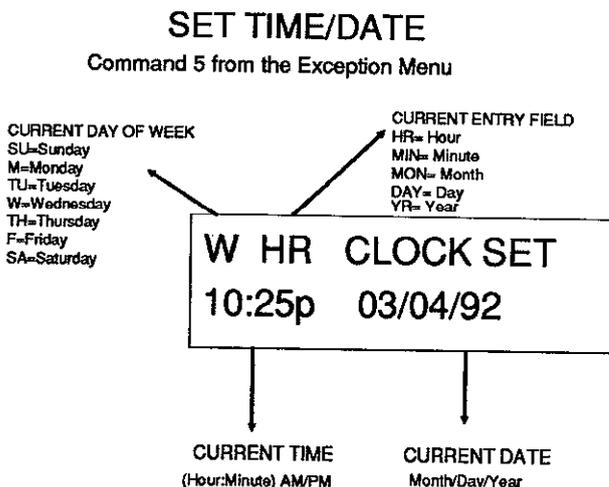
The top line shows the current time and the field being defined. The *INSTANT* key will be used to move between the fields and the *CODE* key is used to change between AM/PM.
