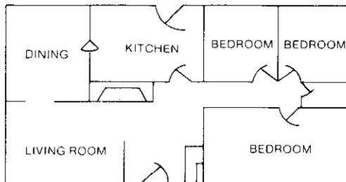
Smoke detector shall be located between the sleeping area and the rest of the house.
