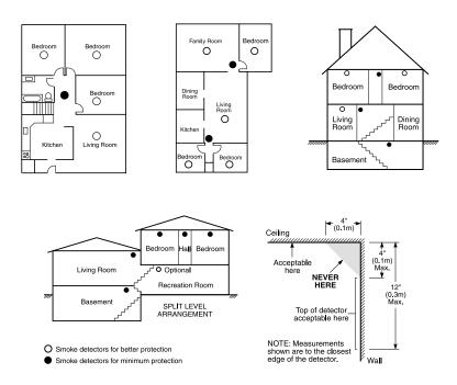
Smoke detectors should always be installed in accordance with NFPA 72, the National Fire Alarm Code. Smoke detectors should always be located in accordance with:
